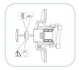
Dismount the old wheel brake disc, nut and mounting cap. Never re-use the old nut and cap.
