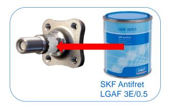
Clean the axle stub from all dirt and pollution. To avoid rust after mounting, always use SKF Antifret (LGAF 3E/0.5) on the stub axle before mounting the bearing.
