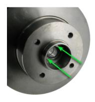
When installing the bearing and the brake disc, apply the force ONLY on the inner ring of the bearing.
