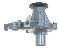
Side profile of the replacement SEM type pump with the front and rear casings pre-assembled.
