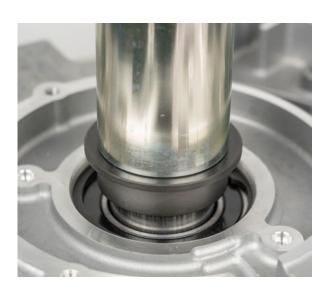
A suitable device must be used to assemble the rotor, such as the Schaeffler E-Axle Repair Tool, to ensure that the rotor and stator do not touch each other
