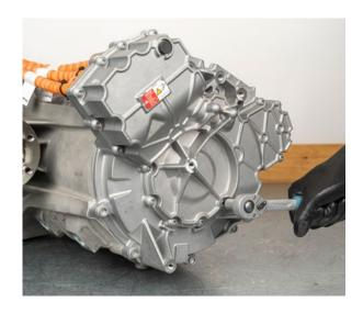
• Loosen the high-voltage cables from the holder
