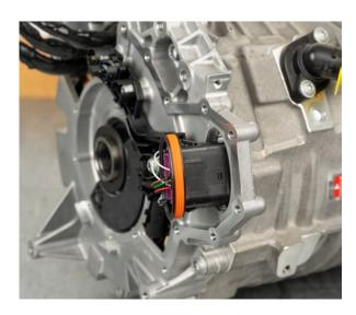
• Disassemble the screws of the rotor position sensor
