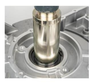
• Press sleeve onto rotor shaft
