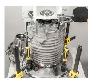
• Remove the thrust washer and spring washer from the transmission-side bearing seat
