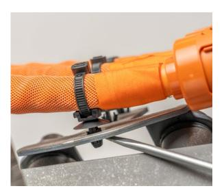
• Remove the screws from the high-voltage cable harness
