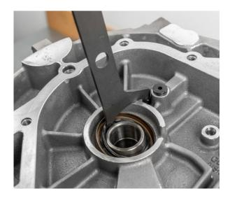
A suitable device must be used to disassemble the rotor, such as the Schaeffler E-Axle Repair Tool, to ensure that the rotor and stator do not touch each other
