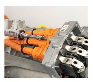
• Mount the high-voltage cables on the high-voltage terminal and tighten the screws to 20 Nm + 45°
