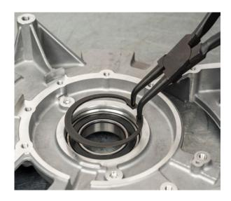
• Pull off the transmission-side bearing
