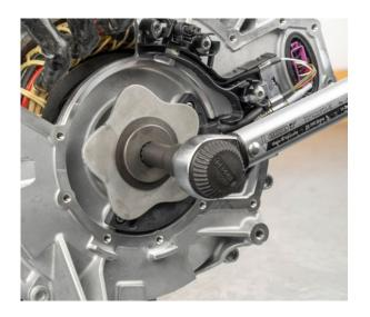
$\bullet$  Install the high-voltage terminal and tighten the screws to 8 Nm + 45  $^{\circ}$
