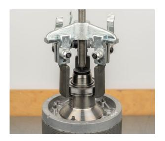
• Press on new transmission-side bearing
