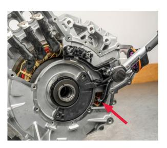
• Insert the screws of the rotor position sensor and tighten to 5 Nm + 90°
