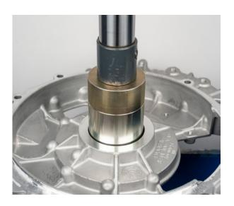
• Press the new motor-side bearing into the housing cover
