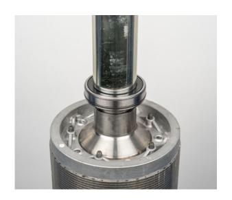
• Press the housing cover with bearing onto the rotor via the inner bearing ring
