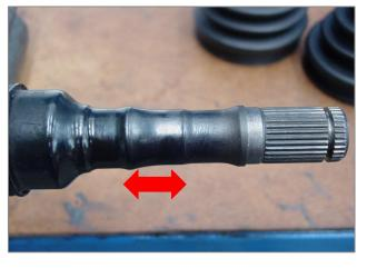
Pic. 4 - Slots for correct boot fitting
