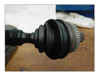
Pic. 3 - Correct position for boot tightening
