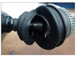
Pic. 2 - Boot cracks due to incorrect tightening
