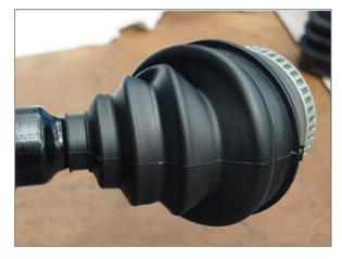
Pic. 1 - Incorrect boot tightening
