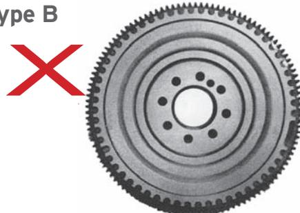
Timing mark differences between the early and later type flywheels will cause non-start of the engine if HKF1001 is fitted to a 'New Transit' model year 2006>
