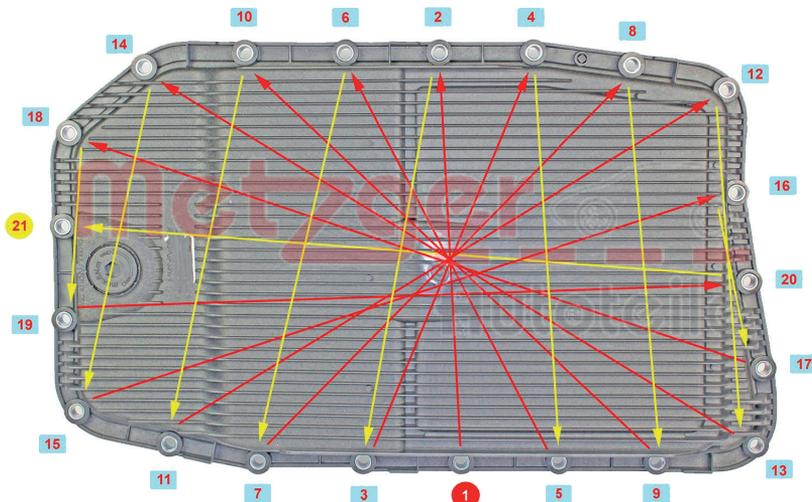
**Tightening sequence:** Keep oil pan on the gearbox and screw all screws in by hand. Check correct fitment of the oil pan. Start fasten screws at position 1 crosswise from inside to outside. Torque 10 Nm. The car manufacturer's instructions must be observed.
