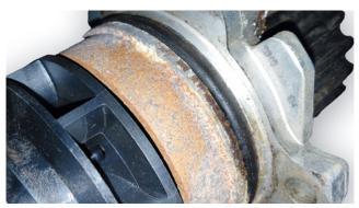
Figure 1: Signs of corrosion on a coolant pump
