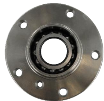
SKF bearing design without outboard seal
