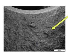
Laboratory examination confirms no fault in the casting
