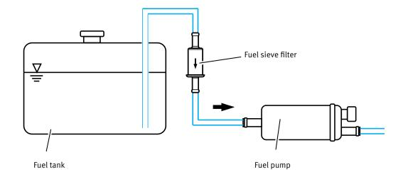
The sieve filters can be installed in the fuel line between the fuel tank and the type E1F fuel pump (with a diameter of 8 mm at the suction nozzle).
