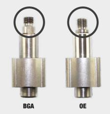
A design flaw in the OE Pump led to insufficient contact area between the drive shaft and the rotor, allowing 3-5° of movement between the shaft and the rotor. BGA reengineered the shaft to increase this surface area by 72%.
