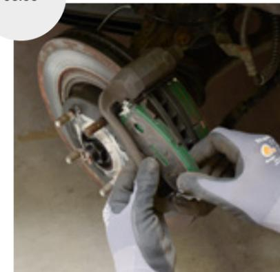
2. Release the brake calliper and remove the brake pads. Attention: when replacing brake discs, always replace the brake pads with them and replace all brake discs/brake pads on the respective axle!
