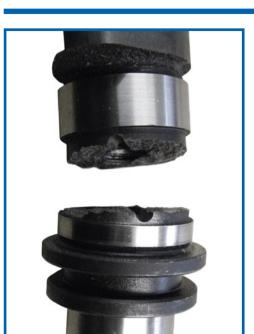
**Appearance:** Camshaft breakage between or through cam-lobes.
