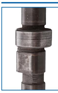
Appearance: Severe cam-lobe wear. Causes: Starvation or contamination of oil, tappet clearance too tight, excessive valve spring pressure. **Remedy:** Thoroughly flush the lubrication system, install new camshaft and followers. Adjust tappets to the correct clearances, prime with extreme pressure lubricant and replace oil and oil filter.
