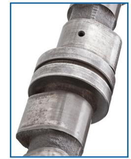
**Appearance:** Severe scoring of the camshaft bearings. Causes: Starvation or contamination of oil, i.e. foreign particles circulating in oil.
