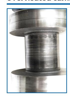
**Appearance:** Cam-lobes, bearings & followers have a 'blue' discoloration. **Causes:** Overheated engine possibly due to
