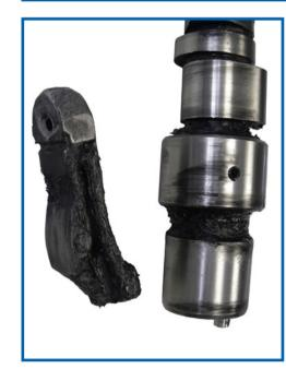
Appearance: Carbonised oil build-up on cam and
