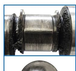
Appearance: Premature wear of one or more camlobes & followers. Follower contact surface will be concaved with chipped edges. Causes: Incompatible cam-lobe & follower contact surface geometry. Often caused by fitting new camshaft with old followers or vice versa. Can also result from lubricant starvation from blocked or restriction in oil
