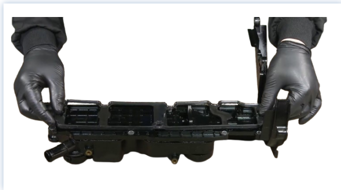
01 | Align and place the gasket in its housing on the cover using the tabs
