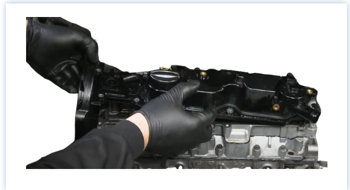
02 | Carefully place the cover on the engine. No sealant should be applied.
