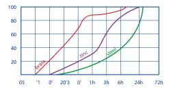
Test Method DIN-54454 Breakaway torque % after immersion
