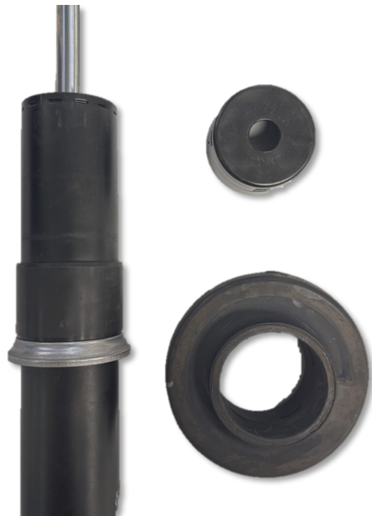
Abb. 4: Federteller demontieren Fig. 4: Removed spring plate
