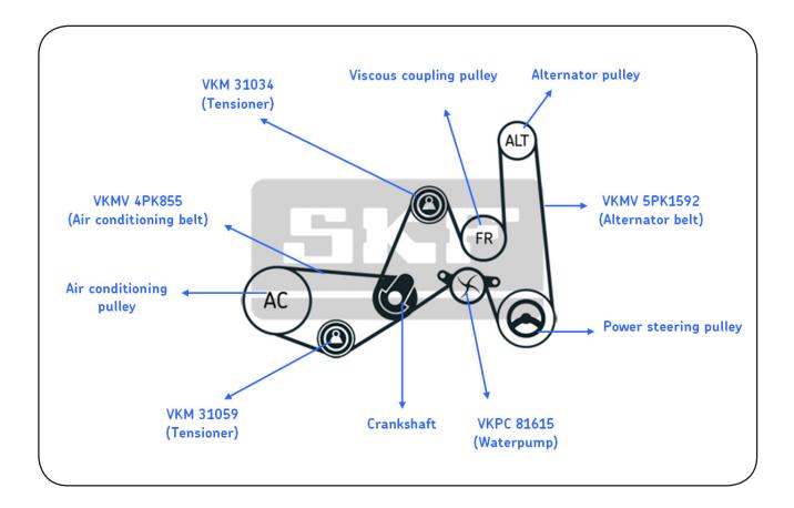
The layout diagram above shows that all of the components (ALT, PS and AC) are driven by the auxiliary belts. That's why we strongly recommended fitting the exact OE belt length when servicing the auxiliary drive system!
