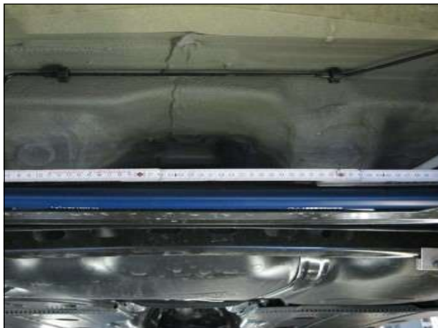
Abb. 1: Messen des Lagergummi Abstands Fig. 1: Measuring the bushing spacing
